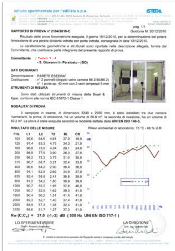
Porta intelaiata spessore 40mm con vetro doppio float. 37dB Rw Framed double glass door 40mm.thick with glass panel in toughened glass 5mm thick => 37dB Rw.
